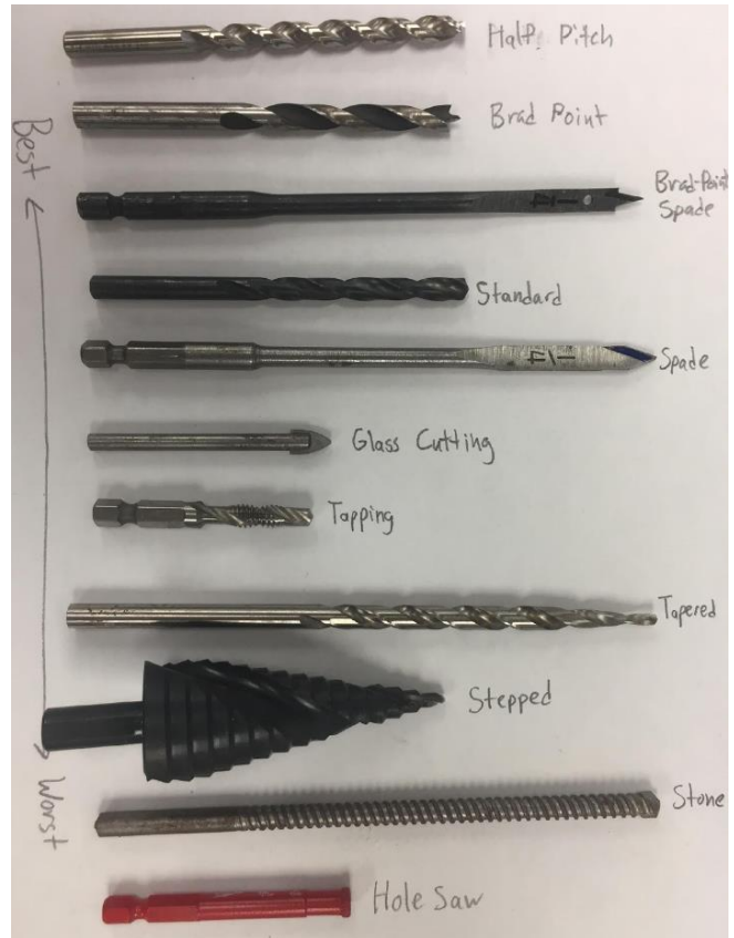
Figure 5: All tested drill bits ranked from least WoB required to penetrate to most.
