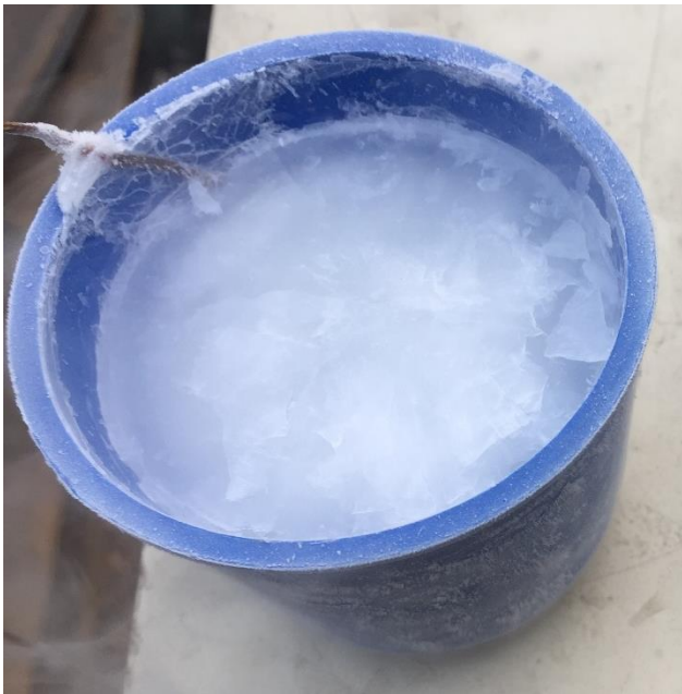
Figure 3: Cryo-ice sample with embedded thermocouple at -180^{\circ}\text{C} before anchoring testing.
