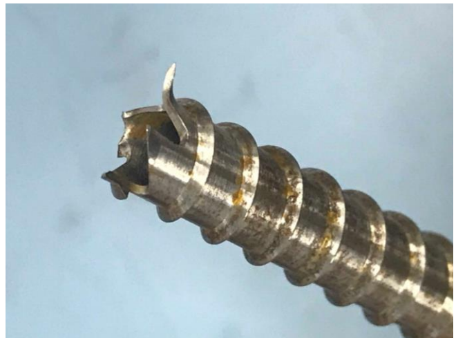
Figure 4: Custom ice screw after cryo-ice testing exhibiting tooth plastic deformation and fracture.
