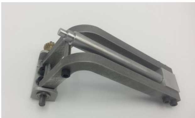
Figure 8: Ice screw clearing mechanism prior to attachment to the ISEE 2.
