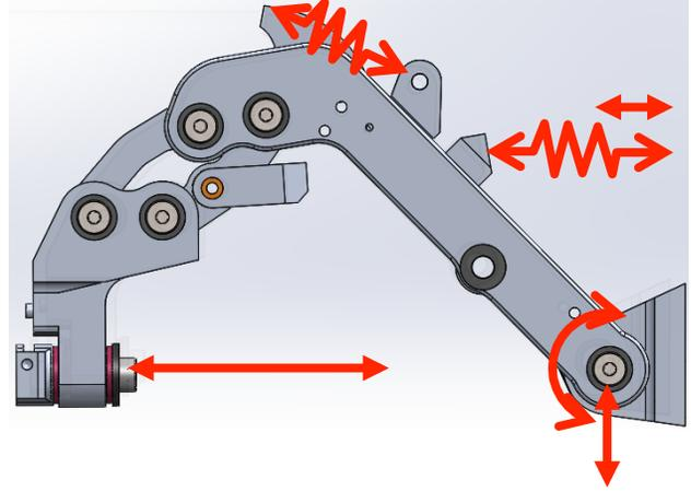
Figure 9: Linkage 3.0 with the six design parameters that will be optimized in the next design.
