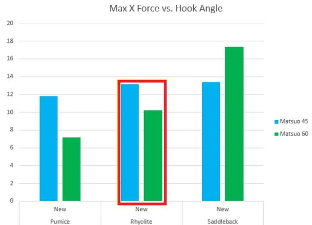
Figure 5: Test results\* of hook angle testing of new Matsuo hooks on different rock surfaces.
