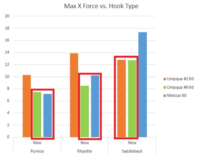
Figure 7: Test results\* of hook type testing of new 60° hooks on different rock surfaces.
