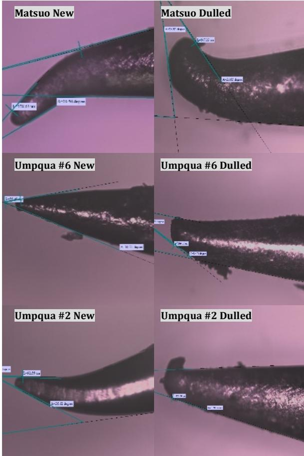
Figure 8: Pictures of microspine tips before and after dulling, taken at 10X zoom.
