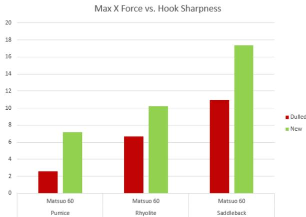
Figure 6: Test results\* of hook angle testing of Matsuo 60° hooks on different rock surfaces.
