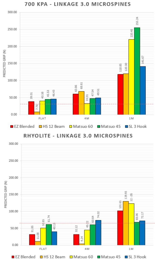
**Figure 4: Test results of flexure testing, showing grip forces on 700kPa Simulant (top) and Rhyolite (bottom) with EZ Blended with Umpqua hooks (red), HS 12 Beam with Umpqua hooks (orange), EZ Blended with Matsuo hooks at 60° (green), and EZ Blended with Matsuo hooks at 45° (blue). The red lines correspond to the WOB requirement for each rock type.**
