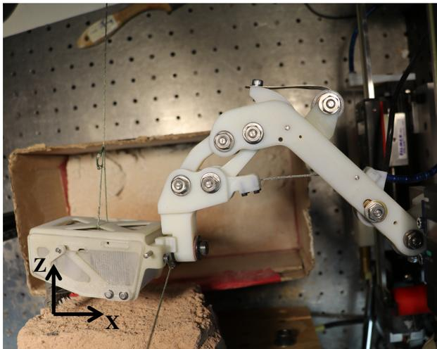
**Figure 2:** A single toe assembly consisting of a linkage (3.0), a cassette of flexures (EZ Blended), and microspines (Umpqua) on the test stand being tested on the surface of a rock sample (Rhyolite).
