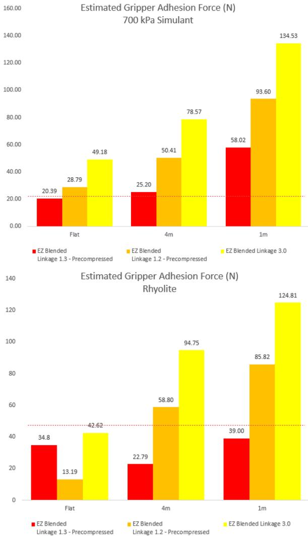
**Figure 3: Test results of linkage testing, showing grip forces on 700kPa Simulant (top) and Rhyolite (bottom) with linkage 3.0 (yellow) outperforming linkage 1.3 (red) and linkage 1.2 (orange) in every case. The red lines correspond to the WOB requirement for each rock type. As shown, even the best performance on flat Rhyolite could not reach the WOB, and performance must be improved to be viable.**
